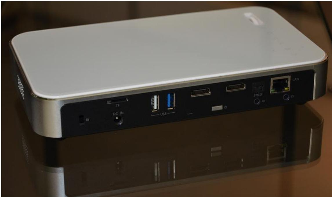
Photo: Inputs: two HDMI with audio, a VGA, an USB and a Micro-SD card slot.
